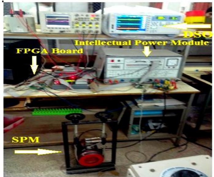
Fig. 20. Experimental Set up of the SPM Drive with FPGA Implementation
